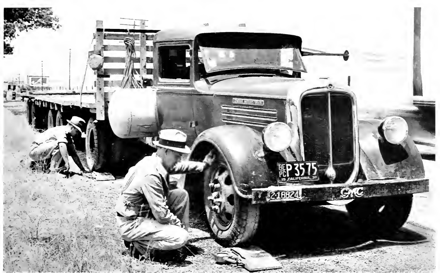
Officials checking weight of large truck and trailer equipment on State Highway. Note portable scales in front of wheels
